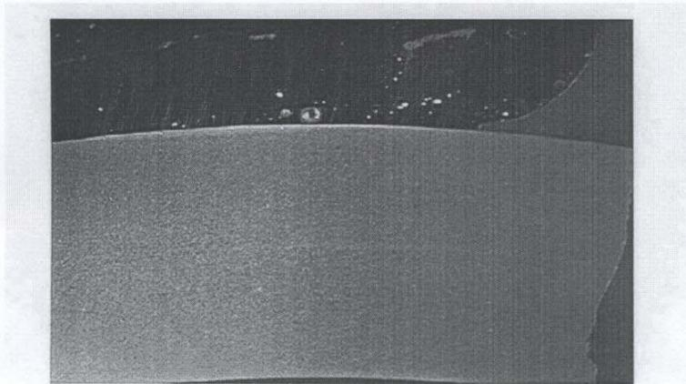
Sample #1 EASYBOND Pin Weld on the base material. Magnification is approximately 9.5X on the original photomicrograph but may be distorted during electronic formatting. Base material is 0.237" nominal and the HAZ (lighter colored area at interface) is essentially negligible. The edge of the pin braze may be seen in the upper right hand corner where the red bakelite meets the curved copper pin
